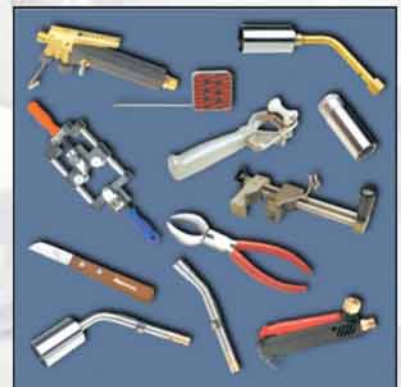
Tool kit for installation/cable preparation
